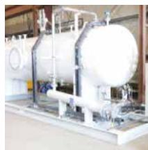
Ammonia Unloading, Storage, Distribution & Vaporization System is designed to provide ammonia (anhydrous or aqueous) reactant to a Selective Catalytic Reduction (SCR) unit for removal of NO<sub>x</sub> from flue gas. Ammonia is delivered by truck or railcar and unloaded into storage tanks. The ammonia is forwarded to the Ammonia Flow Control Unit (AFCU) which generates ammonia gas for injection into the flue gas upstream of the SCR. IFS provides the complete system.
