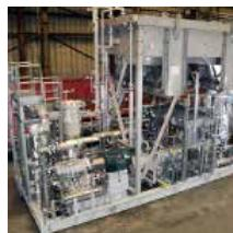
DXP's process capabilities allow us to engineer and build modular gray, blue and green hydrogen generation systems. Hydrogen modules are either build-to-order or engineered to optimize our customer's process requirements (the latter utilizing Aspen HYSIS process simulation software). Whether skid mounted or containerized, our packages are designed as truckable modules for ease in transportation worldwide and minimum site installation time.
