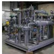
DXP Fuel Gas Conditioning Skids are designed to protect natural gas fueled engines and turbines from liquid slugs, solids (< 0.1 microns) and liquid aerosols. Additionally, the fuel gas is superheated above the hydrocarbon and water dew points to prevent liquid condensation in the turbine's combustion chambers. These systems meet or exceed reciprocating engine and turbine manufacturers' fuel gas quality specifications providing dry, clean fuel to increase the life of the equipment.
