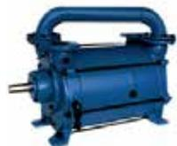
Liquid Ring Vacuum Pumps and Compressors are widely utilized in the biofuel industry. In bioethanol plants, Liquid-Ring Vacuum pumps are used in the distillation and rectification process as well as during the mash liquefaction and drying cycles. By operating under vacuum, the energy consumption of the process is reduced. In the biodiesel industry, liquid ring vacuum pumps and compressors are applied during the separation of biodiesel and glycerine among other filling and emptying applications.
