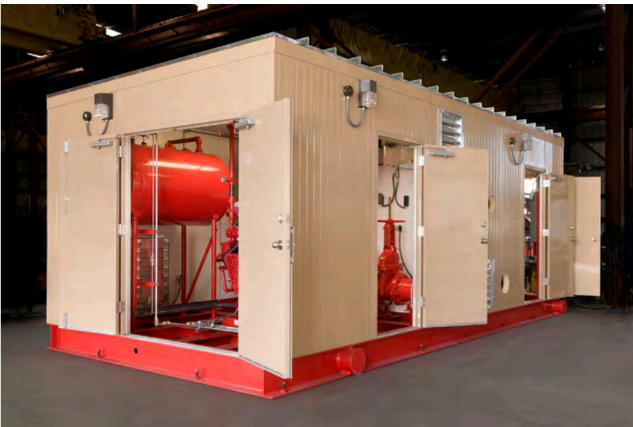
Firewater Pump Package consisting of 2 AC Model 8100 10x8-17F-S horizontal split case pumps, one driven by a 125 HP electric motor with panel, and one driven by a Clarke Model JU6H diesel engine with controller. The package includes an AC 3125 jockey pump and controller; double-walled fuel tank, flow meter, piping, and valves per NFPA 20. Complete package was shipped inside a prefabricated environmental enclosure. Size: 25'L X 12' W X 10'H Dry weight: 30,000 lbs.
