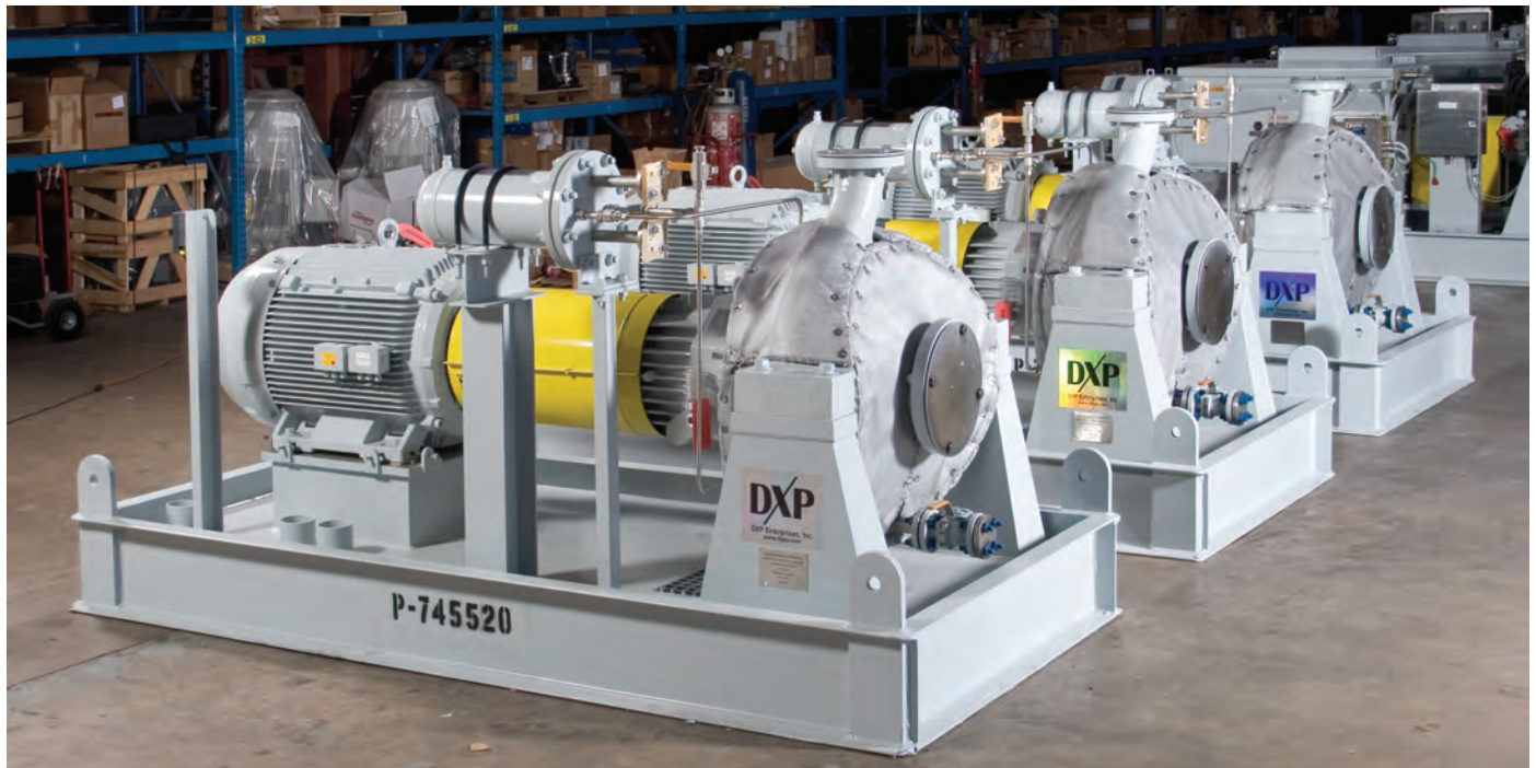
Heat medium circulation pumps, each unit complete with Sulzer model OHH, size 4x8x26, API process pump with heat exchanger, cooled mechanical seals and casing insulation, coupled to an ABB 160 KW, 3000 RPM, 50 HZ, 690 volt electric motor mounted on a custom DXP baseplate.
