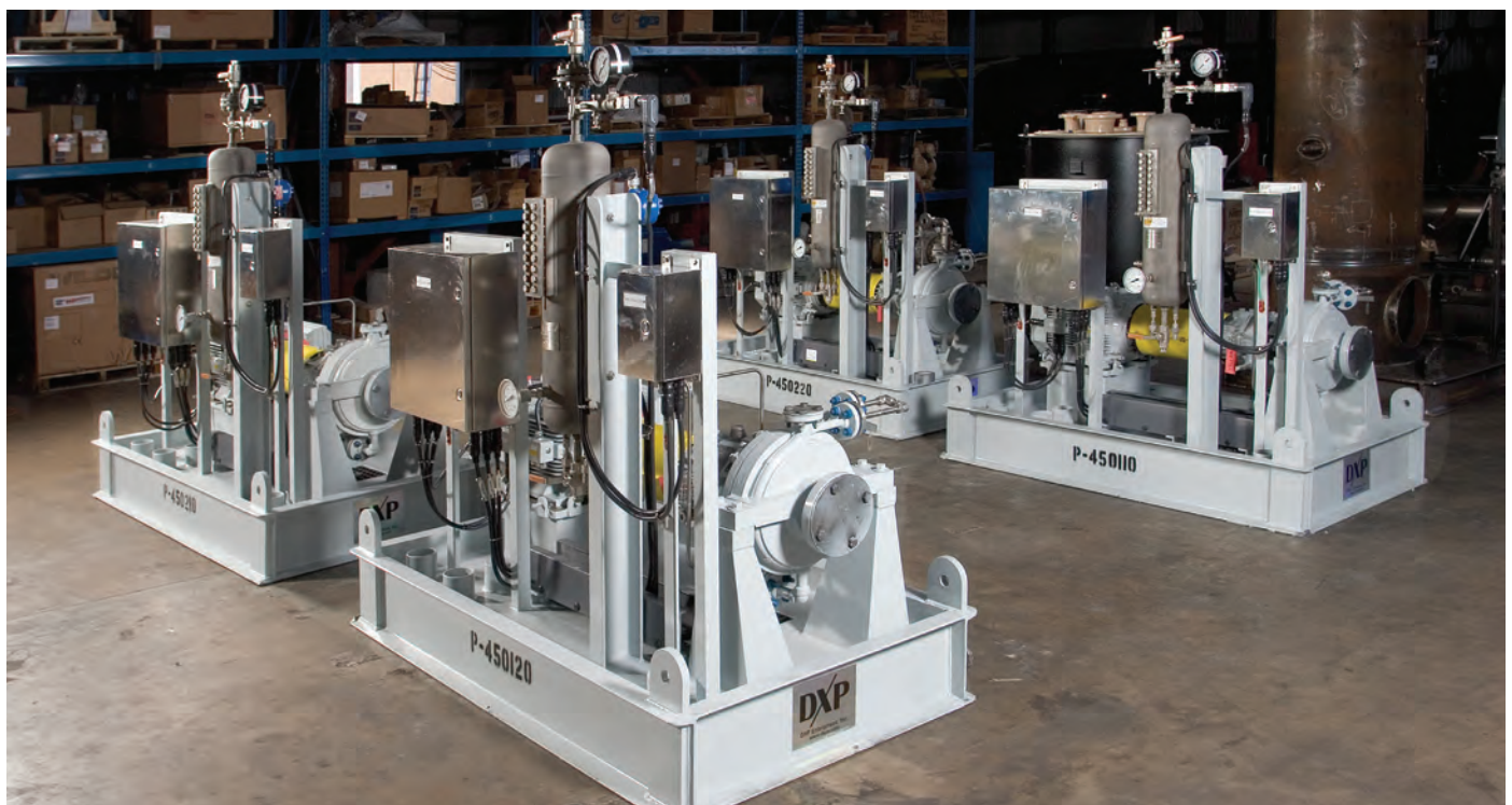
Compression suction scrubber pumps, each unit complete with Sulzer model OHH, size 1x4x14, API process pump with tandem mechanical seal, and API plan 52 seal flush, coupled to an ABB 30 KW, 3000 RPM, 50 HZZ, 690 volt electric motor mounted on a custom DXP baseplate.
