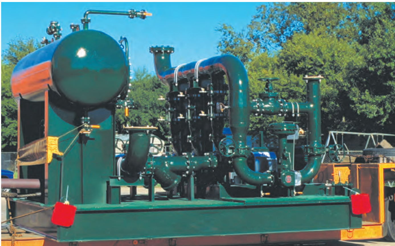
Cooling water skid consisting of three Goulds 3196XLT 6x8-13 ANSI centrifugal pumps driven by 100 HP electric motors and associated pipe, valves, fittings, instrumentation and surge tanks on a common skid.
