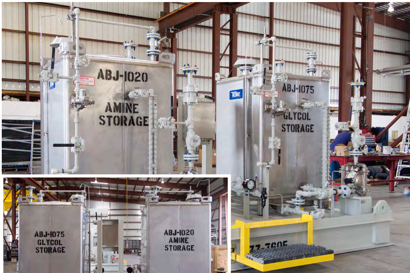
Amine and glycol tank and pump skid consisting of (2) Wilden T4 air operated diaphragm pumps, with control valves, actuated valves, piping and instruments. Dry weight: 6,700 lbs.
