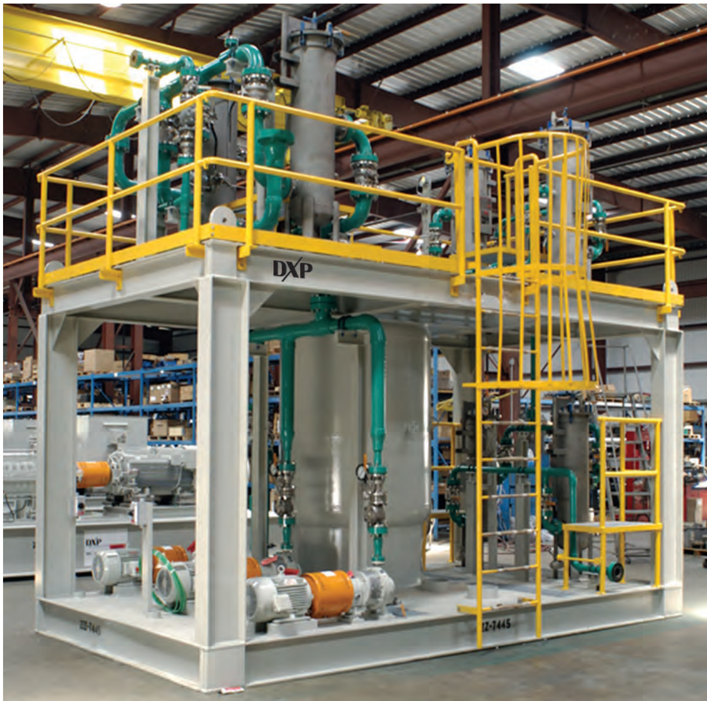
Potable water/pressure set, consisting of three Goulds 3196 ANSI centrifugal pumps. Driven by 20 HP electric motors with associated 316SS valves and filters, Ameron Bondsrand fiberglass piping, and hydro-pneumatic bladder tank on a two-tier skid. Dry weight: 35,000 lbs.
