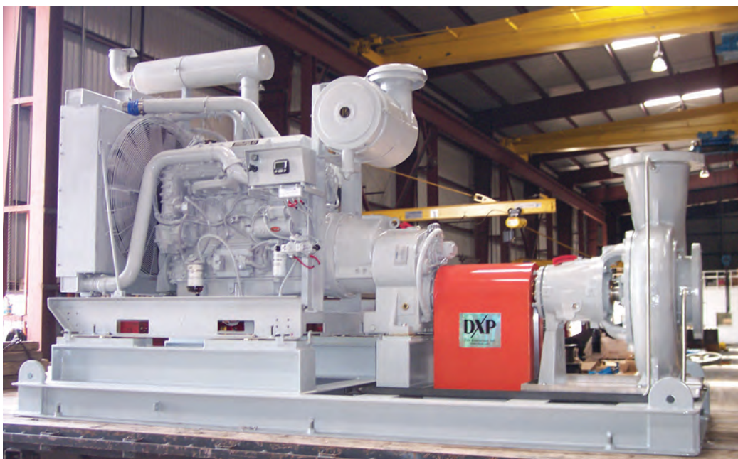
Cooling water skid consisting of a Goulds 3175 14x14-22 pump, driven through a Cotta gearbox, and direct driven by a Detroit 6064 diesel engine. Dry weight: 14,500 lbs.
