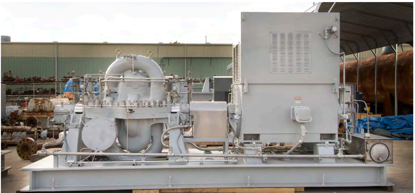
One (1) of twelve (12) PMI skid mounted 1,500 HP mainline pipeline multistage centrifugal pump packages.
