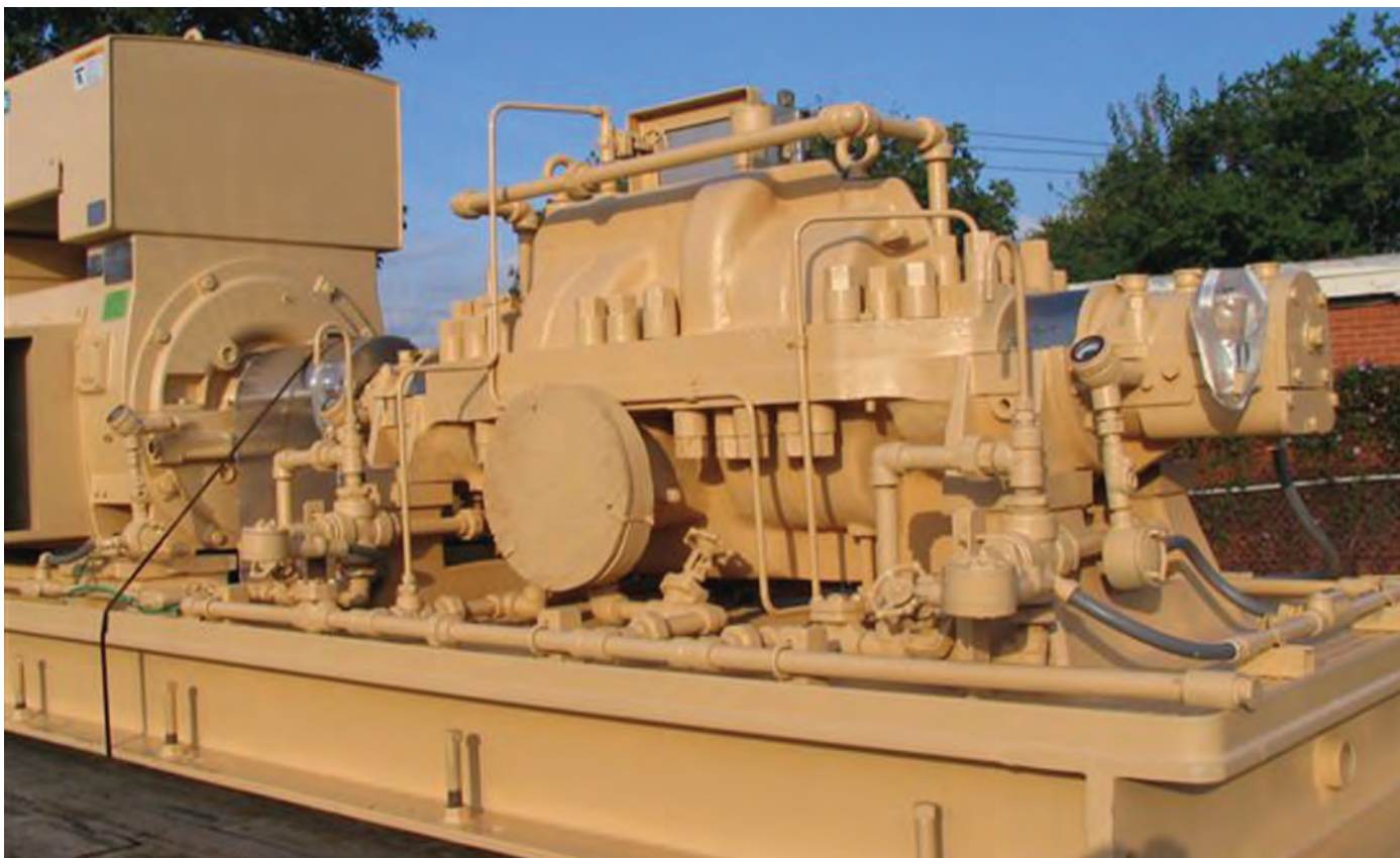
Two (2) PMI hydraulically modified and packaged United N4x11 WMSN, 6 stage heavy duty products pipeline pumps with Siemens 1500 HP, 3600 RPM electric motor drives for 55,000 barrels per day in West Texas. Dry weight: 27,000 lbs. each.
