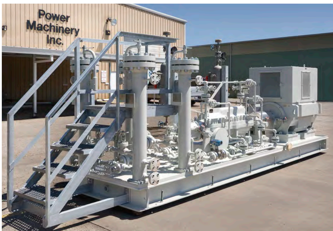
Two (2) remanufactured 400 HP VFD driven Bingham 3x6x9K MSD, 11 stage refinery grade, mixed butane, booster pumps for pipeline application in Mont Belvieu, Texas.
