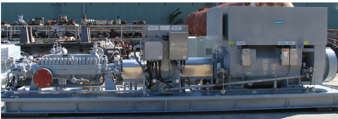
Four (4) PMI hydraulically modified and packaged Bingham 6x6x9K MSD, 10 stage heavy case water injection pumps with Siemens VFD driven from 2,000 HP, 6,600 Volt IEC motors through Lufkin gearbox with speed range at input of 1,200 to 2,000 RPM with output from 3,250 to 5,500 RPM for running in parallel with 7,000 HP units below for 15,000 to 45,000 barrels per day in Chad, Africa. Dry weight: 32,000 lbs. each.
