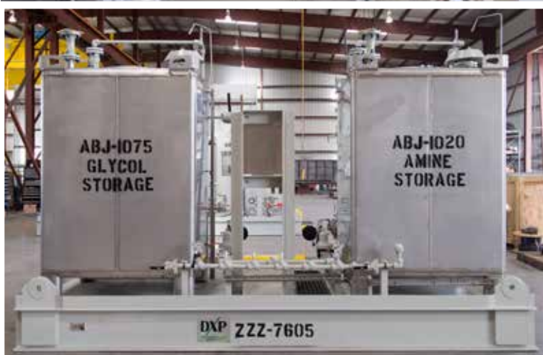
Amine and glycol tank and pump skid consisting of (2) Wilden T4 air operated diaphragm pumps, with control valves, actuated valves, piping and instruments. Dry weight: 6,700 lbs.
