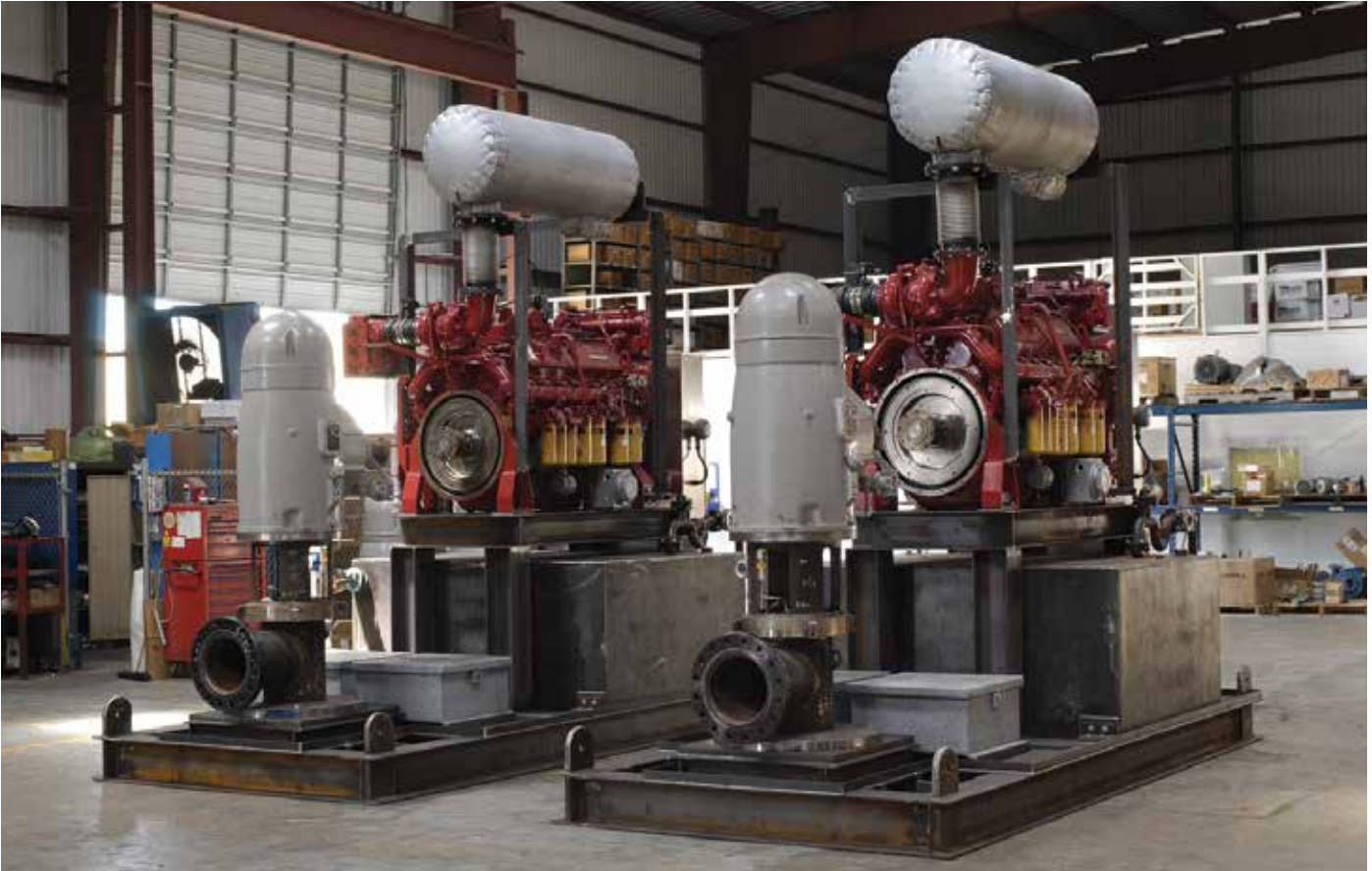
Two firewater pump packages – each package consists of a Goulds 18DMC 4-stage vertical turbine pump, Caterpillar 3412DITA diesel engine, Amarillo S750A right angle gear, and 12" fabricated discharge head. Dry weight: 15,748 lbs. each.
