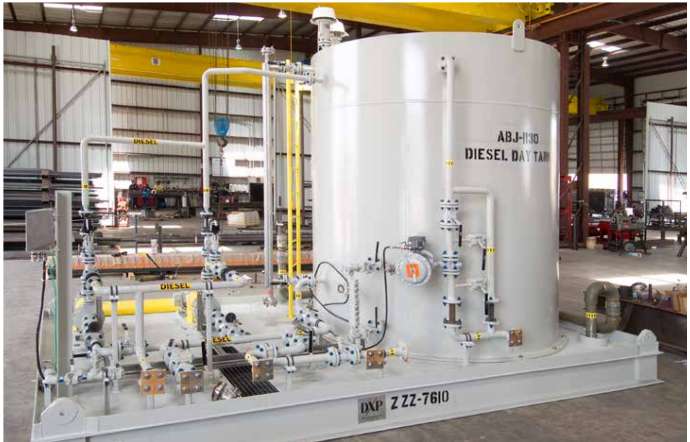
Diesel day tank skid package consisting of a 3600 gallon carbon steel tank with (2) Goulds LF3196 STX, 1x1½ - 8, 316SS centrifugal pump direct driven by a G.E. 3HP, IEEE, 841, electric motor. Unit includes piping valves and instruments. Dry Weight: 15,600lbs.
