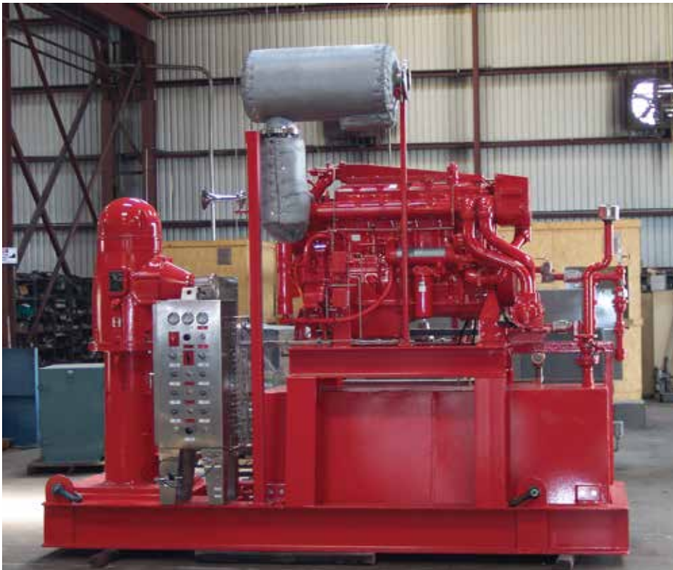
Firewater pump package consisting of two Goulds horizontal split case pumps, 3408 8x10-20L and 3409 8x12-20L with Caterpillar 3406 engines. Included on the same skid was a Goulds 3410 2x3-11, 60HP wash down pump and a G&L SSV jockey pump. Complete package with piping and controls per NFPA 20. Dry weight: 38,000 lbs.
