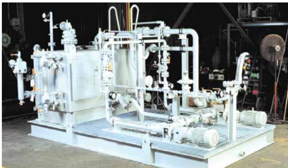
Drain tank skid consisting of (2) Seepex model 5-24 BN progressive cavity pumps driven by 7.5 HP electric motors with associated pipe, valves and fittings, and drain tank on a common skid.
