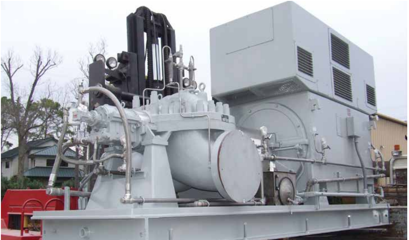
One of two PMI hydraulically modified Bingham 14x14x21 KX HSB single stage, heavy duty, centrifugal, pipeline booster pumps for pumping 240,000 barrels a day (7,000 GPM) @ 1,400 feet of gasoline in a single stage requiring 3,000 HP @ 3,560 RPM. Dry weight: 31,075 lbs. motor and skid.
