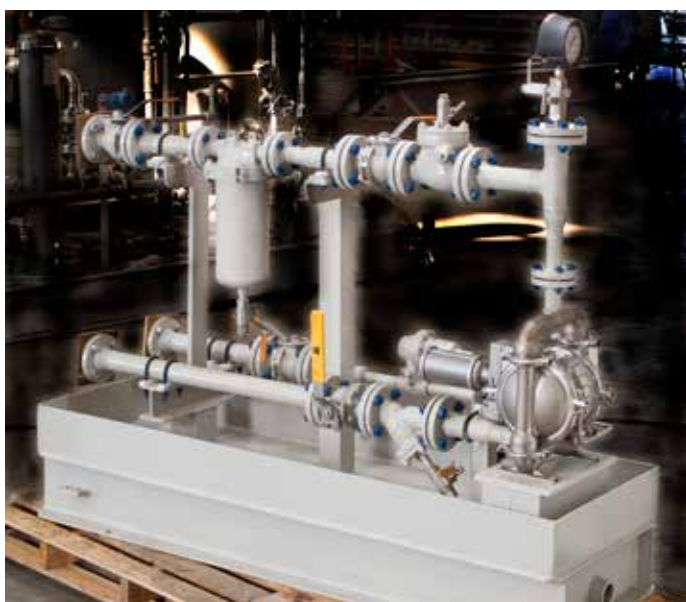
Diesel transfer package consisting of a stainless steel Wilden PV4 air operated diaphragm pump with piping, valves, and filter for suction and discharge lines. Mounted on a common skid with 6" curbing. Dry Weight: 725lbs.
