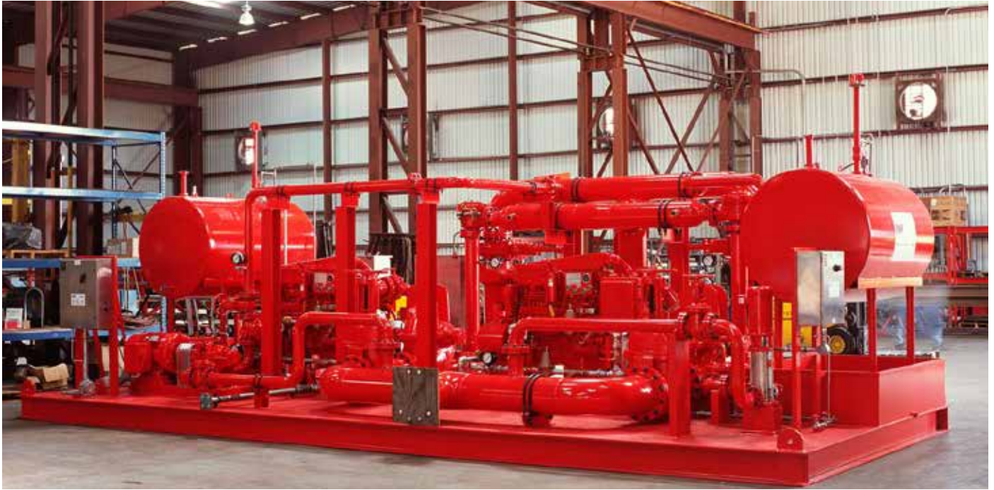
Firewater pump package consisting of two Goulds horizontal split case pumps, 3408 8x10-20L and 3409 8x12-20L with Caterpillar 3406 engines. Included on the same skid was a Goulds 3410 2x3-11, 60HP wash down pump and a G&L SSV jockey pump. Complete package with piping and controls per NFPA 20. Dry weight: 38,000 lbs.
