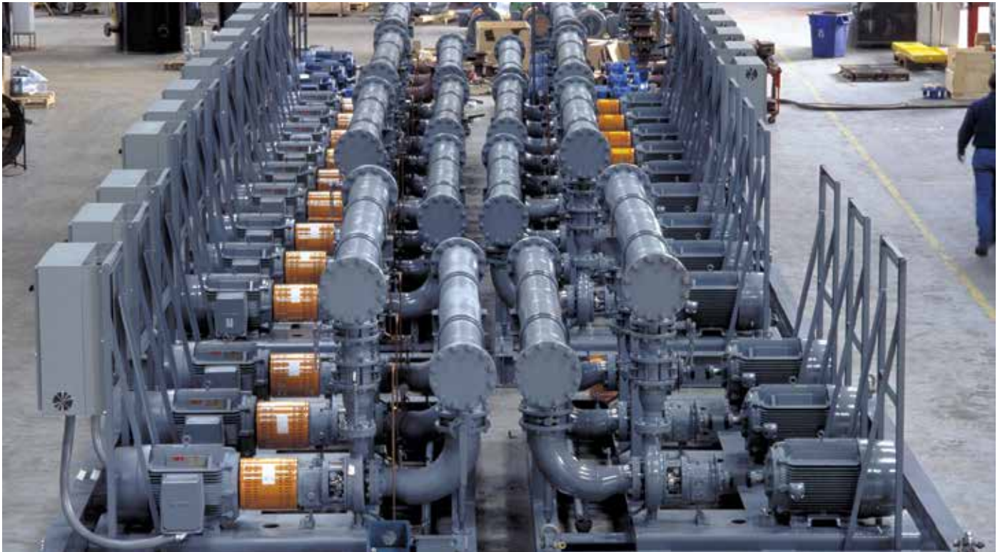
Cooling water skids each consisting of three Goulds 3196 LTX 4x6-10G ANSI centrifugal pumps driven by 100 HP electric motors with TB Woods AC inverters and associated pipes, valves and fittings on a common skid. Dry weight: 11,680 lbs.
