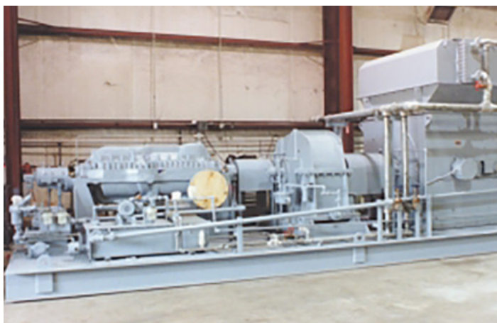
PumpWorks remanufactured Union MQE coke cutter pump, gearbox, lube system and 3000 hp, 6000 V, 50 Hz motor. Unit remanufactured and shipped in 10 weeks.
