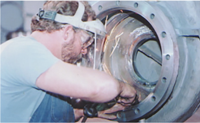
| Single stage casing being reworked to match impeller for hydraulic rate.
