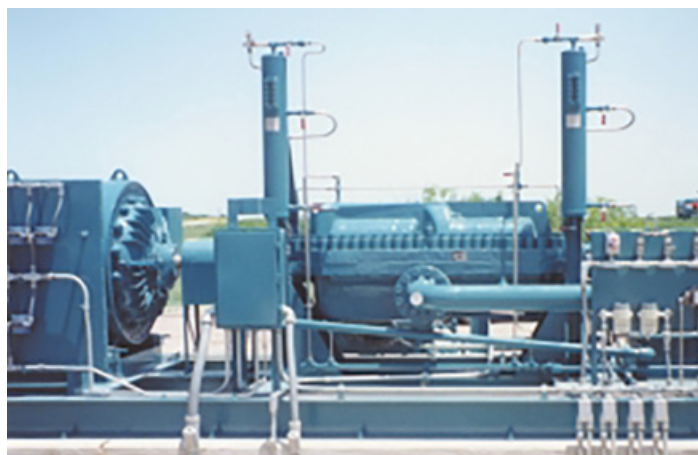
PumpWorks remanufactured Bingham MSD 6X8X11D -10 stage for natural gas liquid, 0.49 spgr. Pipeline application. Unit complete with tandem seals, plan 52, lube oil system and 800 hp motor. Unit shipped in 12 weeks.
