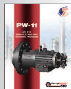
PW-11 is the PumpWorks 610 retrofit upgrade kit for any brand of API 610 single stage OH2 process pump. See our PW-11 API 610 Upgrade Program Brochure for more information.
